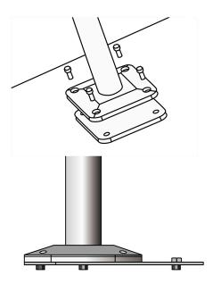
Now you are ready to install the Pedestal Unit. Carefully place the Pedestal Unit over the conduit and wires.
