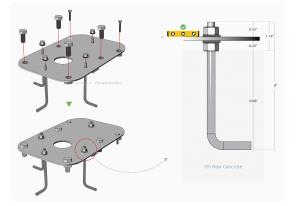
Insert the anchor plate into the concrete (Figure-8).
