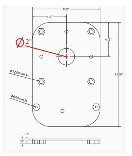
Fit all J-Bolts (4), Pedestal (4) and CMS (2) Disposable Bolts to the anchor plate. (Figure-6)
