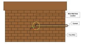
NOTE: If the conduit is run on the same side of the wall as the charging station the wires are then run through the 1-inch opening on the side of the Wall/Pole Mount Bracket Post.
