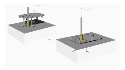
Note: Continuously check for the anchor plate until concrete sets to make sure that anchor plate does not sink into the concrete
