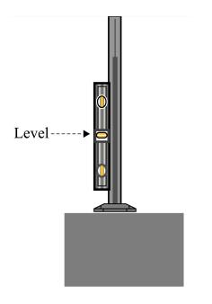
First insert anchor bolts and secure with one or two turns, but do not tighten.
